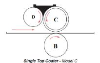
In our *Model C Coater Roll Configuration*, the water base adhesive is held in the trough between the coating roll and its companion doctor roll, top only.
